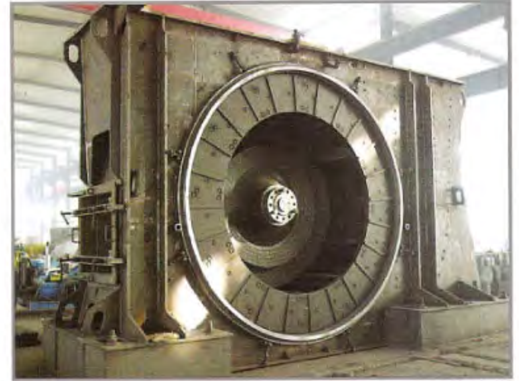
风扇磨煤机 Beater wheel mill
