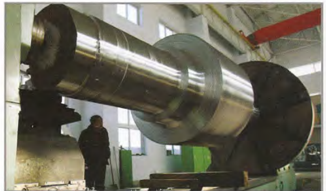
辊轴加工中 Roller shaft under machining
