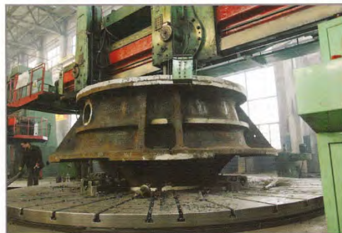
旋回破碎机壳体加工中 Gyratory crusher shell under machining
