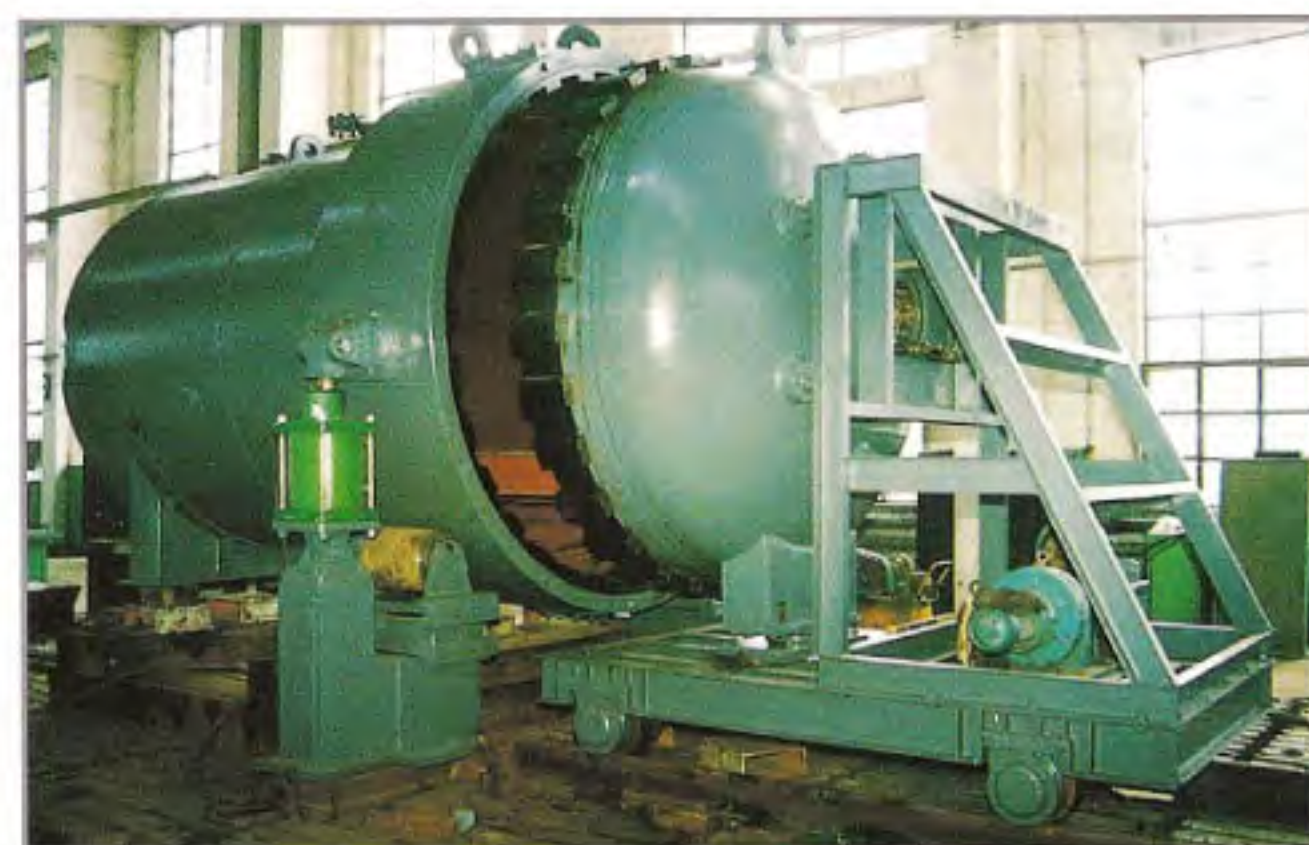
防爆罐 Explosion-proof container
