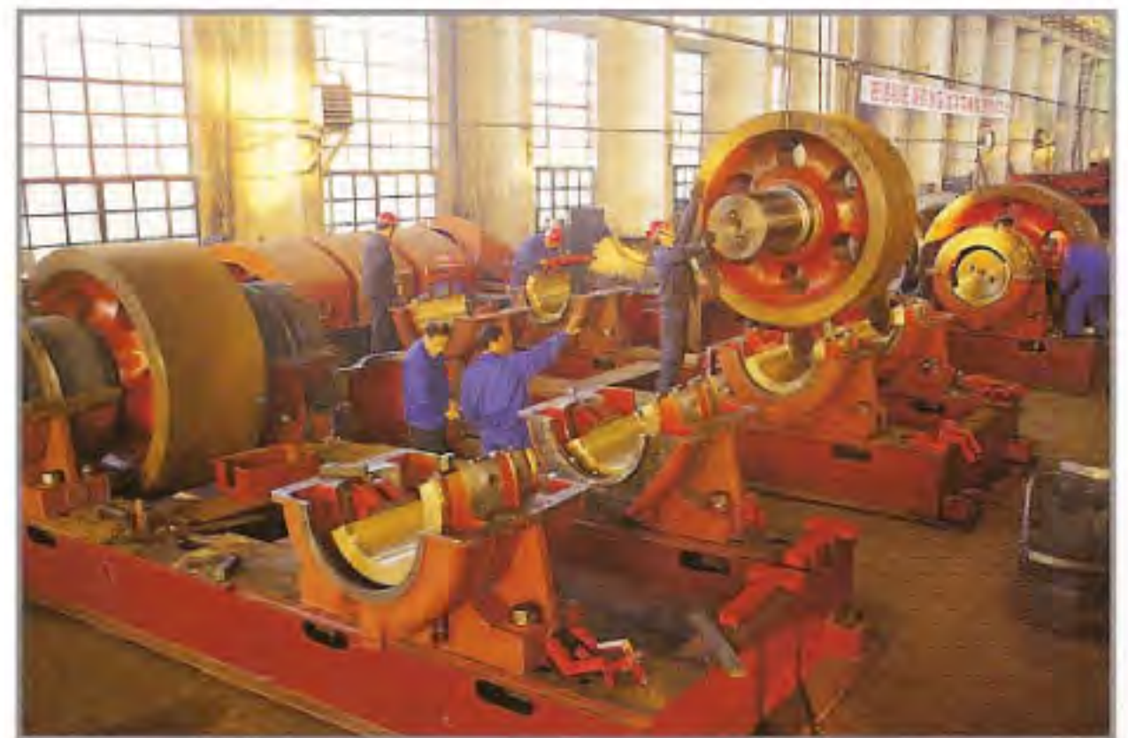
日产5000吨窑支撑装置在装配中 Support device of 5000tpd kiln under installation
