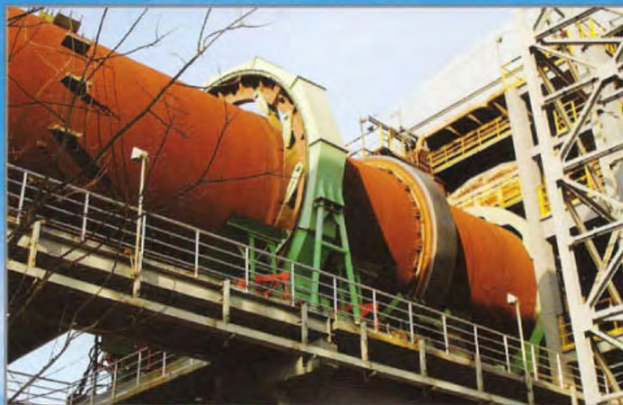
\Phi 6.1 \times 40\text{m} 冶金球团回转窑 (鞍钢) Metallurgical pellet kiln
